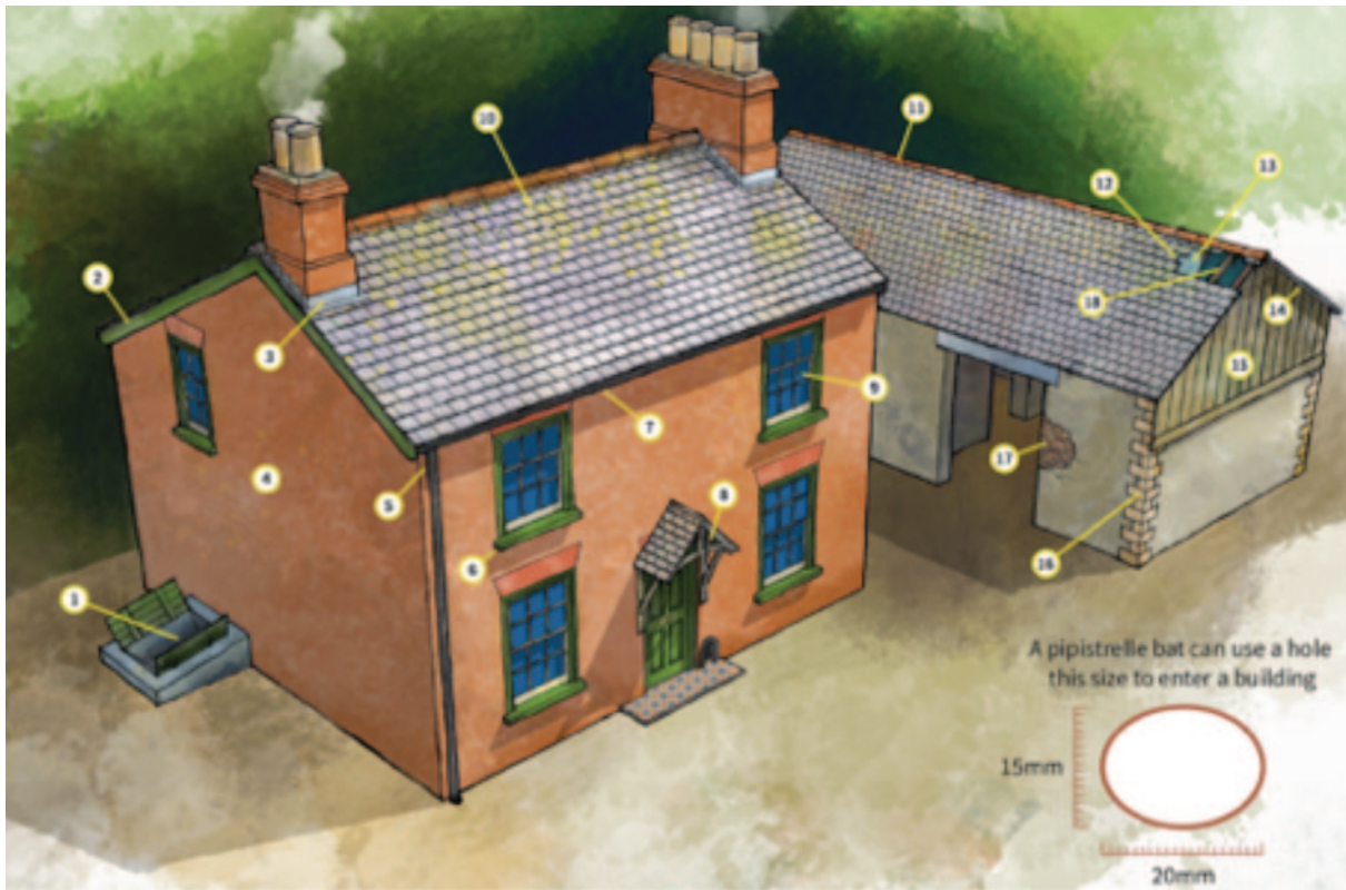
Figure 5.2. illustrates places where bats frequently roost (© Historic England with the permission of BCT) 69 .
